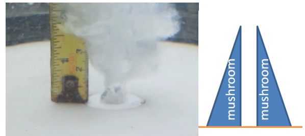
Fig.4. The shape of the ice accretion.
